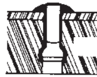
GROOVED RIVET Grooves improve holding strength
